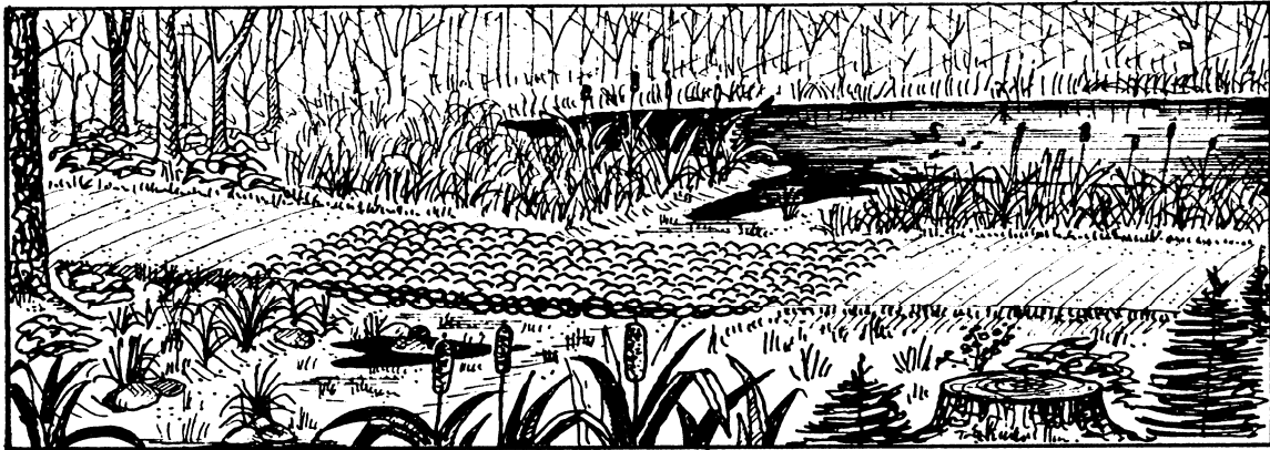
Figure 37. Stone ford crossing over low-lying channel: suitable only on limited use camp roads.
