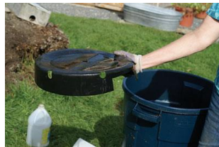
Fig 5. Cut notch in drain pan to fit over handhold recess & connector
